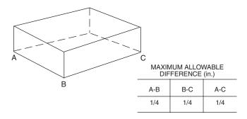
Fig. 3 - Unit Leveling Tolerances
